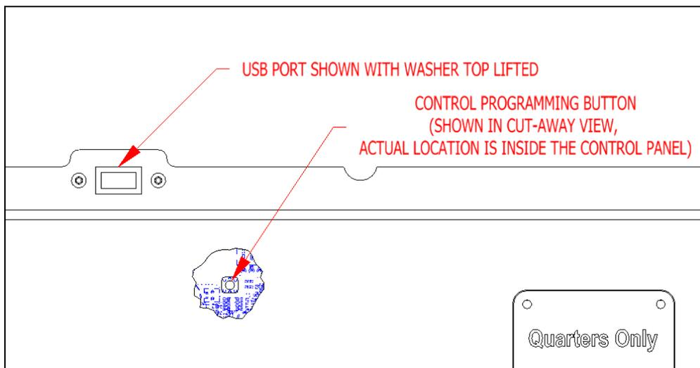
When manual programming mode is entered, the "Start", "Hot", "Warm" and "Cold" buttons perform alternate functions.
