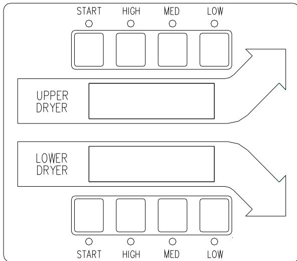
Both dryers are operated by the controller at the left midpoint of the dryer. The controller is two-in-one with the upper display and lights dedicated to the upper dryer and lower display and lights dedicated to the lower dryer.
