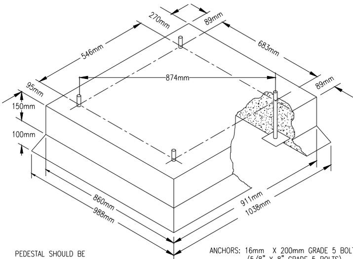
PEDESTAL SHOULD BE REINFORCED WITH MESH OR RODS.
