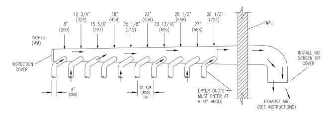
FIGURE 3— Dryer Exhausting Using A Main Discharge Duct.
