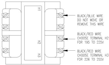
Figure 2 CONTROL TRANSFORMER CONNECTIONS
