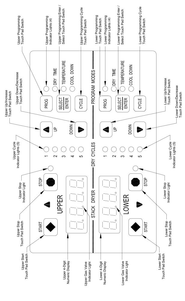
Figure 4: Non-Reversing Dryer Controller Interface
