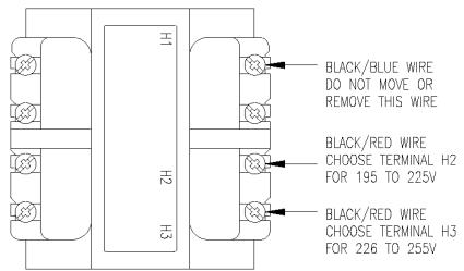
Figure 3 CONTROL TRANSFORMER CONNECTIONS
