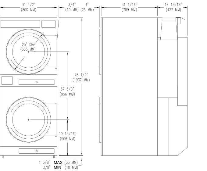
Figure 1a, 30# Stack Dryer Dimensions, inches (mm)
