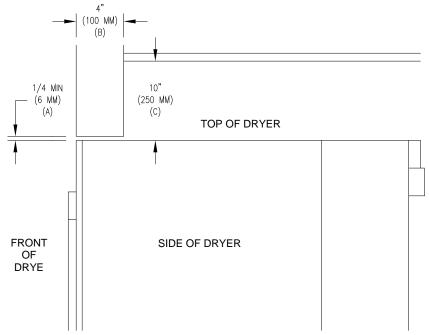
FIGURE 2 Vertical Clearance Dimensions
