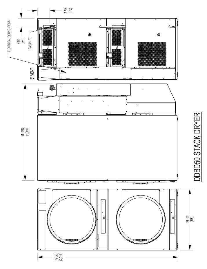
Figure 1b, 50# Stack Dryer Dimensions, inches (mm)
