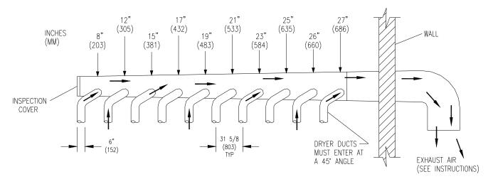
FIGURE 3- Dryer Exhausting Using A Main Discharge Duct.
