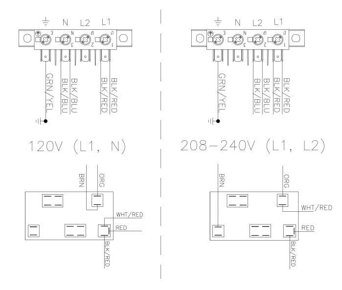
6. Move the black/red wire from the 120V tap on the transformer found in the bottom of control box to the required voltage tap based on actual supply voltage measurement. See figure below.
