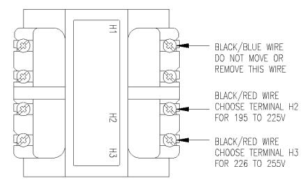
Figure 3: CONTROL TRANSFORMER CONNECTIONS
