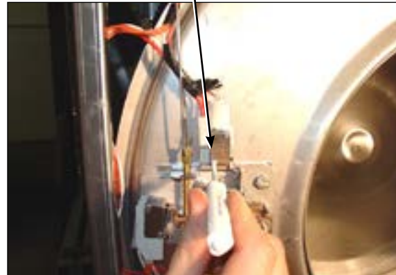
Flat blade screw on door switch latching
