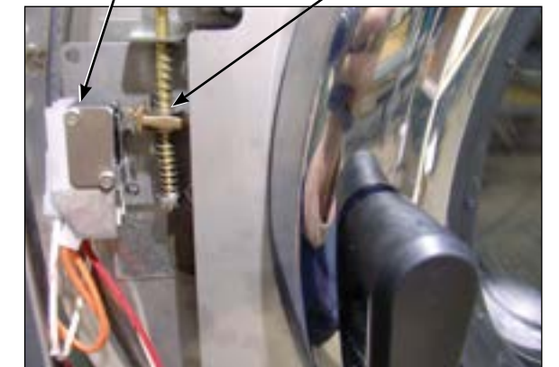
Top of flat end of locking pawl.
