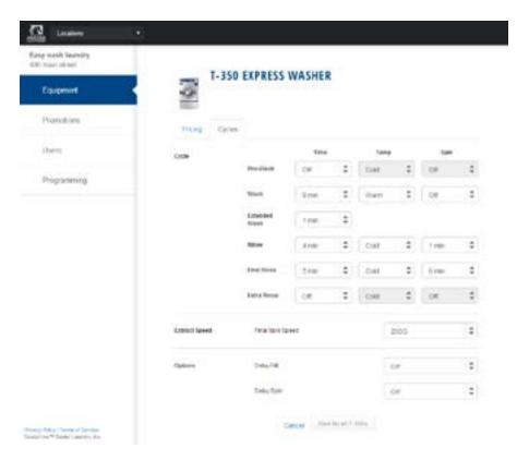
Adjust cycle programming set the length of time and extracts speed as needed.
