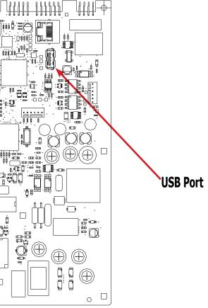
CAUTION!!! Be sure that any loose keys or other items that are connected to the USB device are removed from the USB stick to prevent any possible metal contact
