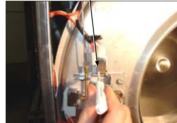
Flat blade screw on door switch latching
