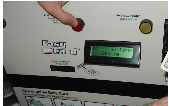
Step 4: Insert a dollar bill from the front side of the cabinet and press the red button.
