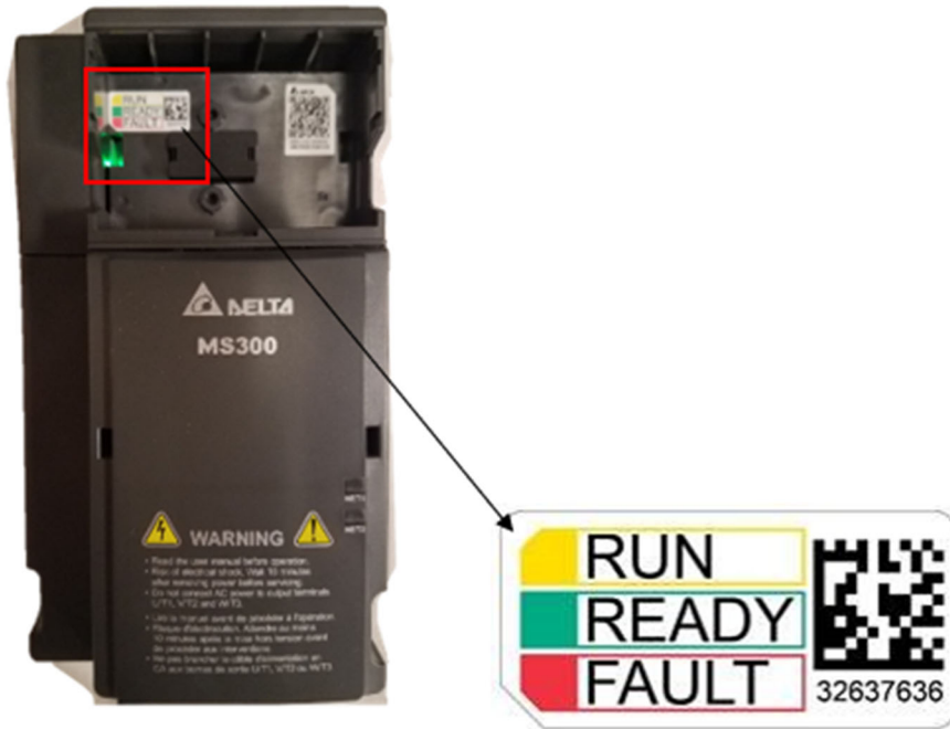
Figure 7-34 VFD Indicator LEDs
