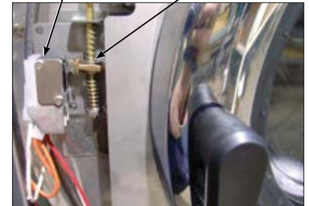
Top of flat end of locking pawl.
