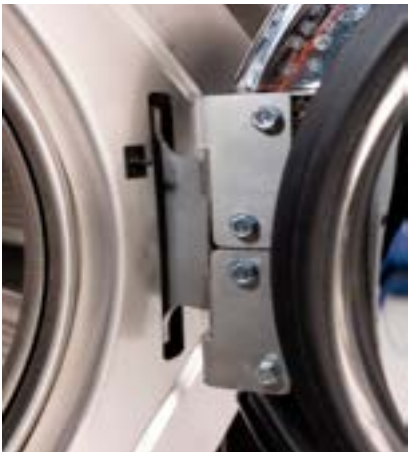
Step 2: Remove 2 bolts holding the lower leaf hinge and set door off.
