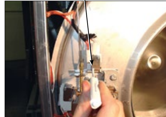
Flat blade screw on door switch latching
