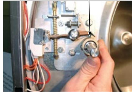
**Step 4:** Check for switch actuation at partial turn of cam as in operation above. Door handle goes from horizontal to six o'clock vertical.
