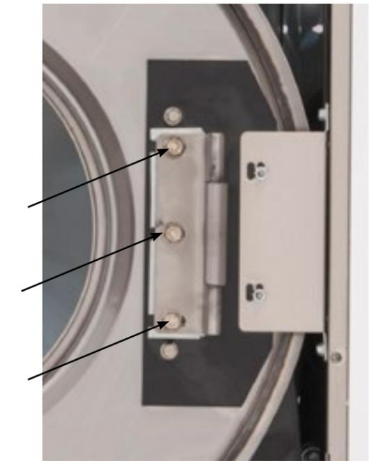
**Step 2:** Remove 3 screws holding door hinge. Shims may be present between hinge and tub front. The number may be increased or decreased to adjust right side door pressure.
