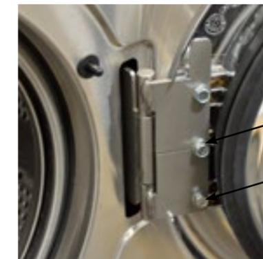
**Step 2:** Remove the bottom 2 bolts holding the lower leaf hinge and then remove it. The door can now be lifted from the upper post of the hinge assembly.
