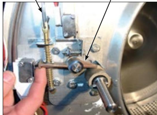
**Step 5:** Check that lock pawl arm swings to cam lobe to lock position.
