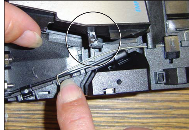
Move spring downwards to free the catch.
