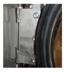
**Step 2:** Remove 2 bolts holding the lower leaf hinge and set door off.
