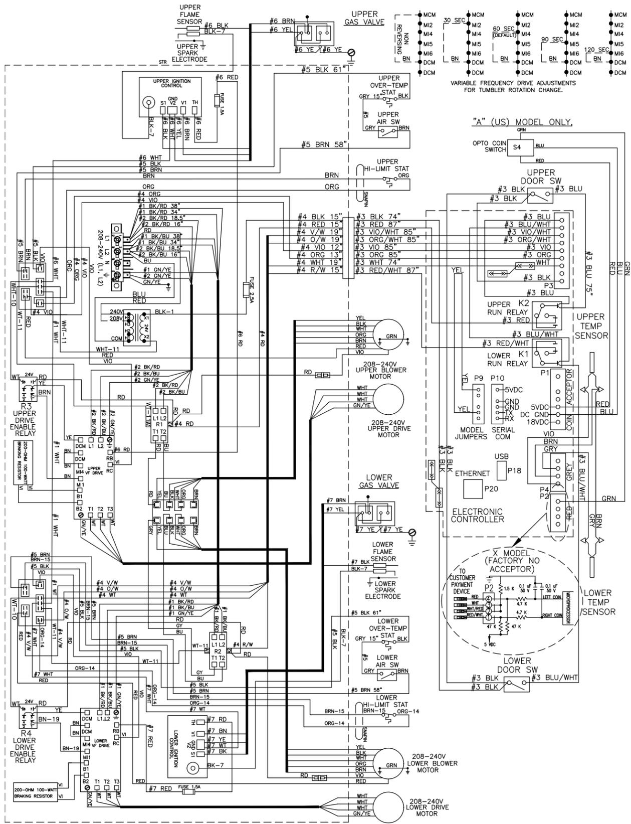
9506-790-001B WIRING DIAGRAM DC50X2NC-11EC\_R
