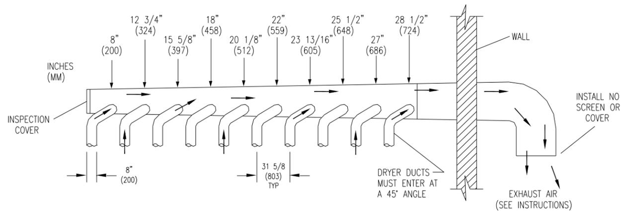
**NOTE:** A small diameter duct will restrict airflow; a large diameter duct will reduce air velocity - both contributing to lint build up. An inspection door should be provided for periodic clean out of the main duct.
