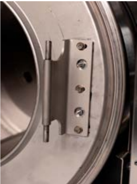
Step 2: Remove 3 screws holding door hinge. Shims may be present between hinge and tub front. The number may be increased or decreased to adjust right side door pressure.
