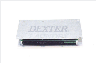
30-CYCLE CONTROL (CPU) BOARD 9799-002-003
