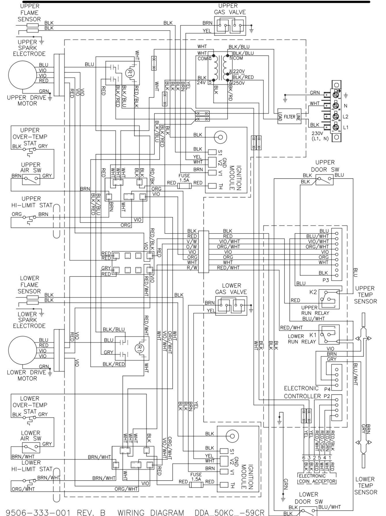
9506-333-001 REV. B WIRING DIAGRAM DDA\_50KC\_-59CR
