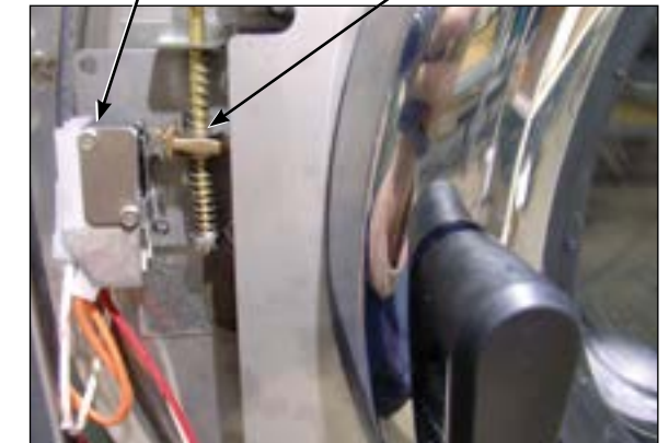
Top of flat end of locking pawl.
