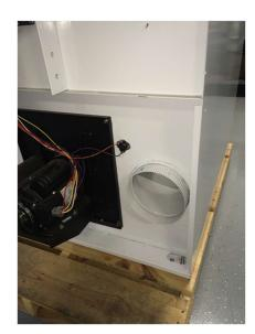
3) Remove factory exhaust outlet (may require drilling out rivets).
