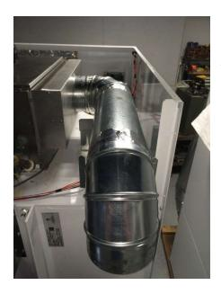
6) Assemble duct onto machine as shown with (2) screws through the burner housing recirculation inlet into the recirculation duct.
