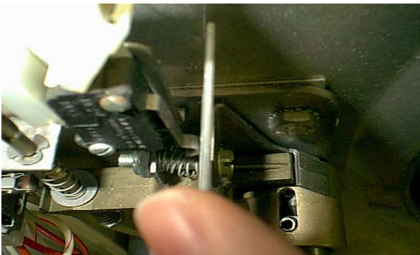
PHOTO # 3 SHOWS GUAGE IN PLACE FOR ADJUSTMENT
