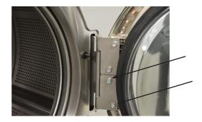
**Step 2:** Remove the bottom 2 bolts holding the lower leaf hinge and then remove it. The door can now be lifted from the upper post of the hinge assembly.
