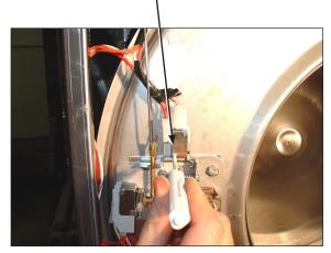
**Step 3:** With switch actuator bracket adjusted you will now need to adjust single switch by loosening 2 flat brade screws and allowing swivel of switch. Move switch towards above bracket until it actuates. Now tighten flat blade screws. Use a .040 thickness guage to insert between bracket and switch and the switch should close and open again upon removal of thickness guage.
