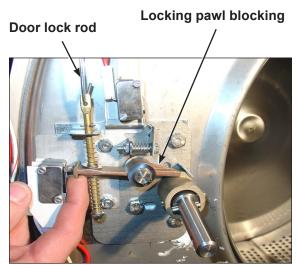
**Step 5:** Check that lock pawl arm swings to cam lobe to lock position.
