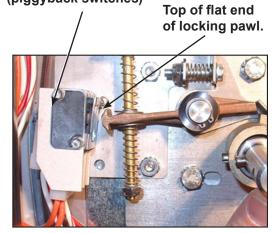
**Step 6:** The lock stacked switches (piggyback) must be adjusted as door lock solonoid pulls up on door rod and locking pawl is now blocking door cam from turning and is in full up position. The stacked swtiches (piggyback) have a single actuator arm and it must actuate when single actuator roller wheel rolls to flat side of locking pawl. You will also notice a .040 gap between actuator arm and switch bodies.
