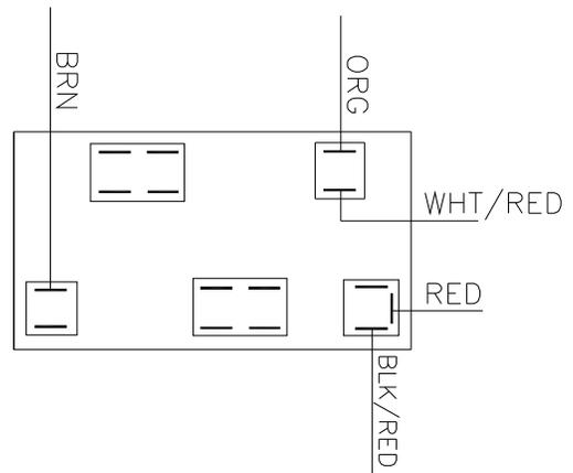
6. Move the black/red wire from the 120V tap on the transformer found in the bottom of control box to the required voltage tap based on actual supply voltage measurement. See figure below.
