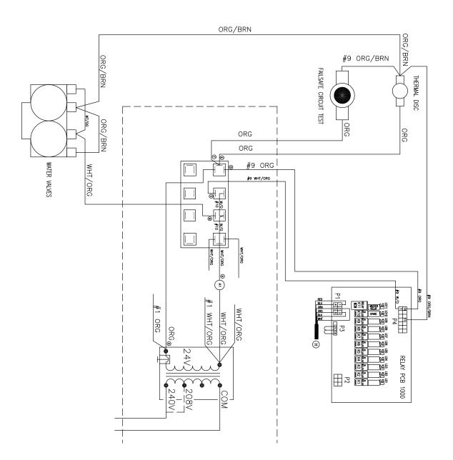
WIRING OF THE FSS SYSTEM USING THE SAME TRANSFORMER AND TERMINAL BLOCK FROM SHEET 1
