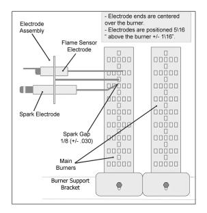
6. However,at the end of 3 separate retries of 10 seconds "Trial for Ignition", the flame is not established, the ignition system goes into "Safety Lock-Out" and will not reactivate the "Trial for Ignition" until there is a current interruption for a period of 15 seconds. This interruption can be provided by opening the dryer loading door and allowing the machine to come to a complete stop for 15 seconds.
