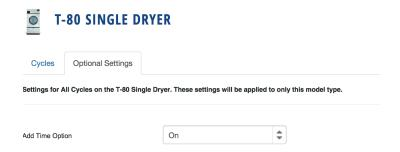
DexterLive can control time adjustment options for the end user. Turning Add Time off would restrict users from adding time once a cycle is complete or during a cycle.
