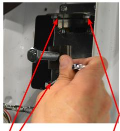
Right side adjustment nut tighten First.
