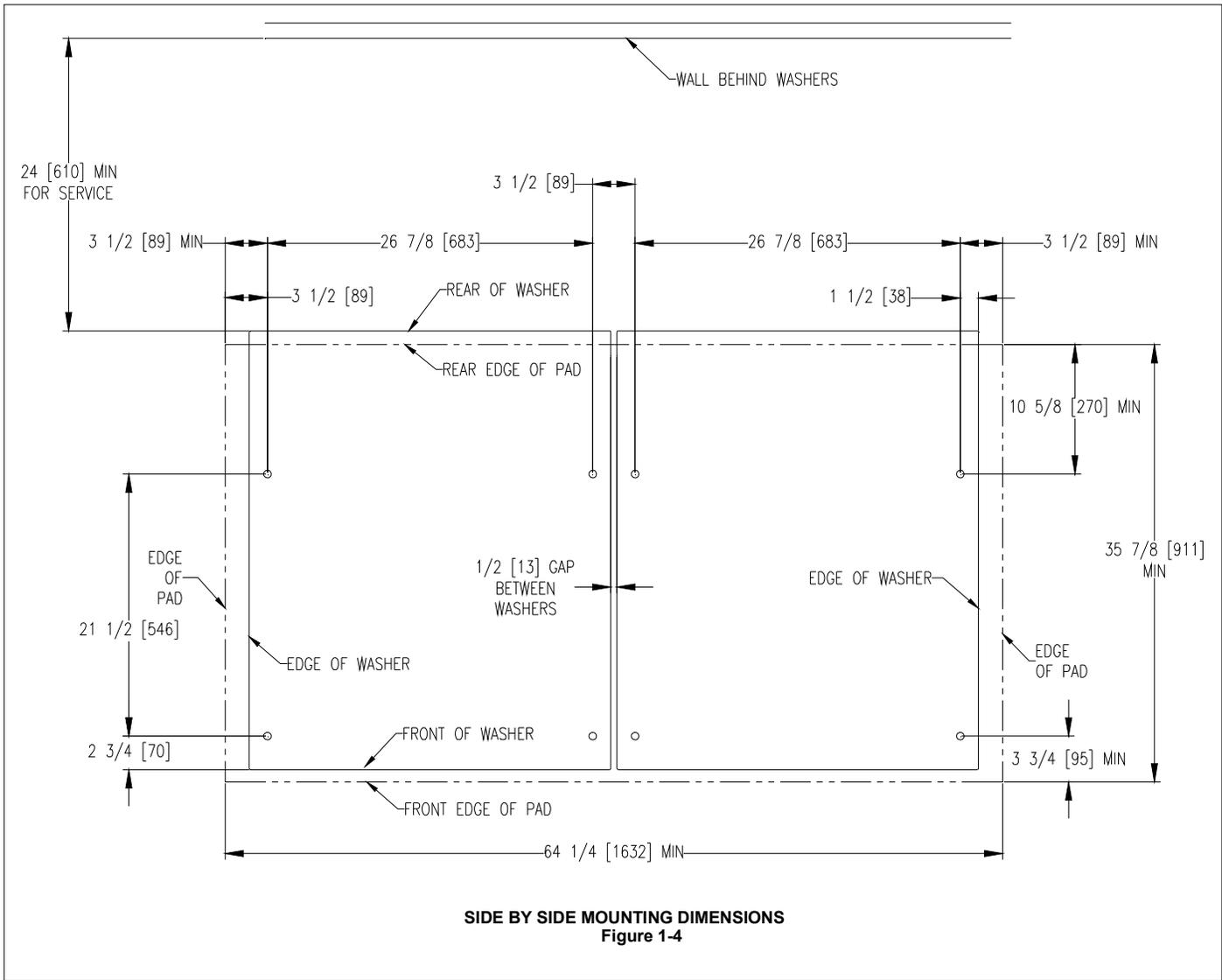
***T-600 Machine Side By Side Mounting Detail***
