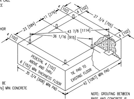
PEDESTAL SHOULD BE 4,000 PSI [28 MPa] MIN CONCRETE REINFORCED WITH MESH OR RODS.
