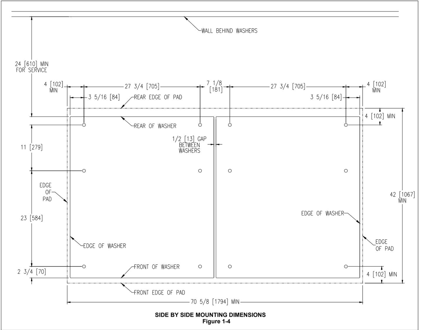
***T-900 Machine Side By Side Mounting Detail***
