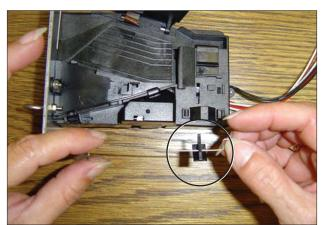
Attach the plastic part to the new spring.
