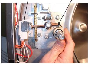
Step 6: The lock stacked switches (piggyback) must be adjusted as door lock gear motor pulls up on door rod and locking pawl is now blocking door cam from turning and is in full up position. The stacked switches (piggyback) have a single actuator arm and it must actuate when single actuator roller wheel rolls to flat side of locking pawl. You will also notice a .040 gap between actuator arm and switch bodies.
