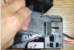
Rotate the spring clockwise for about 40 to 60 degrees until it becomes free of the protrusion. Lift off the spring with the attached plastic part.
