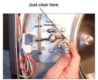
**Step 1:** Set door cam over pin. Here you can see the door cam away from the door lock assembly.
