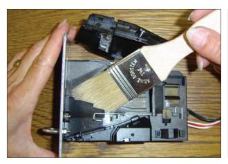
Clean the coin path with a soft brush and wipe the exposed surfaces. Use an alcohol moistened cloth.
