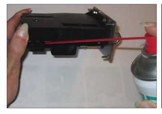
Optical sensors may be cleaned with a soft brush or very carefully with an air spray duster.
