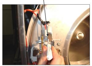
Step 3: With switch actuator bracket adjusted you will now need to adjust single switch by loosening 2 flat blade screws and allowing swivel of switch. Move switch towards above bracket until it actuates. Now tighten flat blade screws. Use a .040 thickness gauge to insert between bracket and switch and the switch should close and open again upon removal of thickness gauge.
