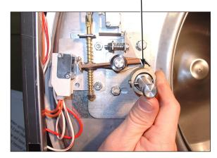
**Step 4:** Check for switch actuation at partial turn of cam as in operation above. Door handle goes from horizontal to six o'clock vertical.
